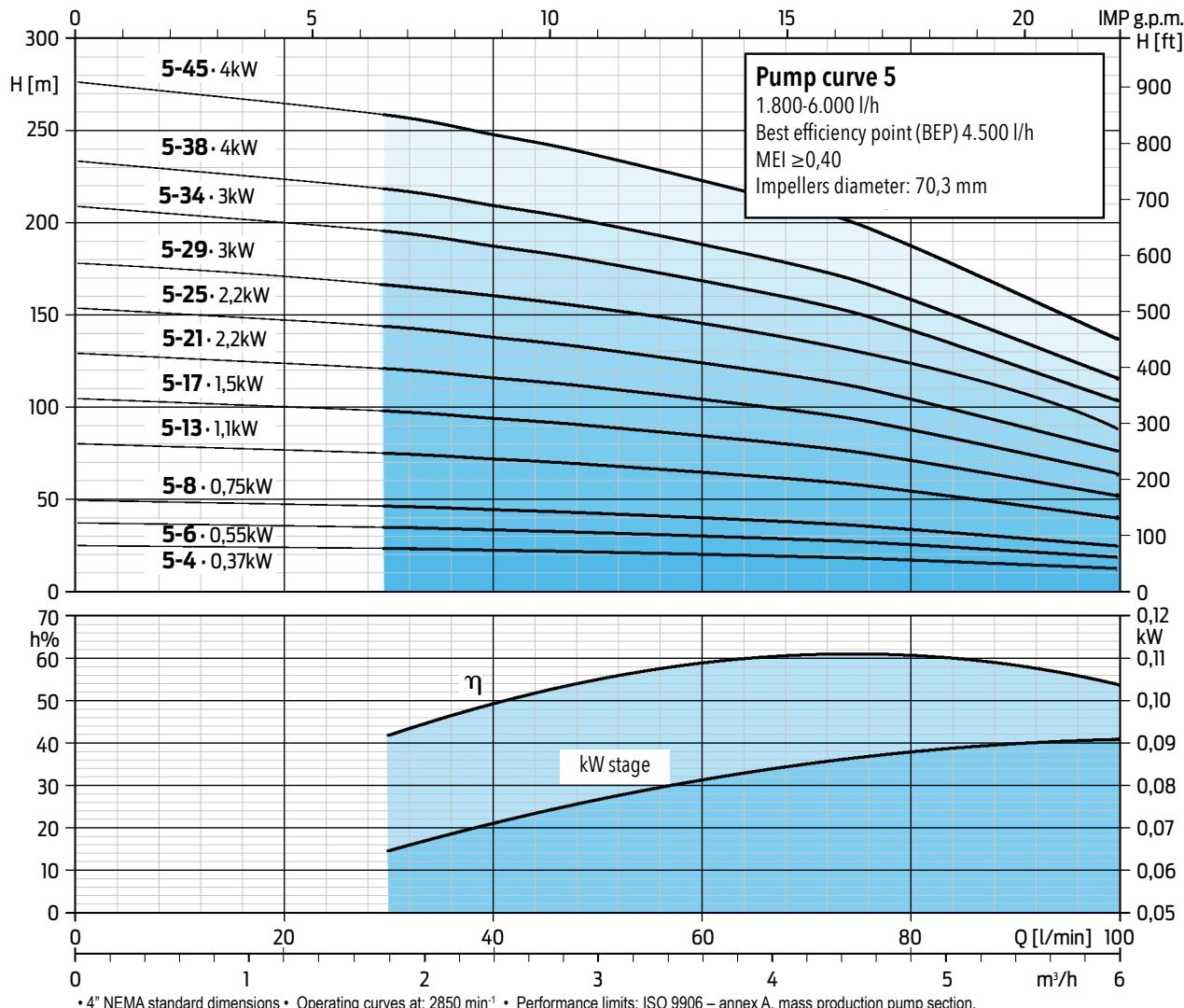
• 4" NEMA standard dimensions • Operating curves at: 2850 min<sup>-1</sup> • Performance limits: ISO 9906 – annex A, mass production pump section.
