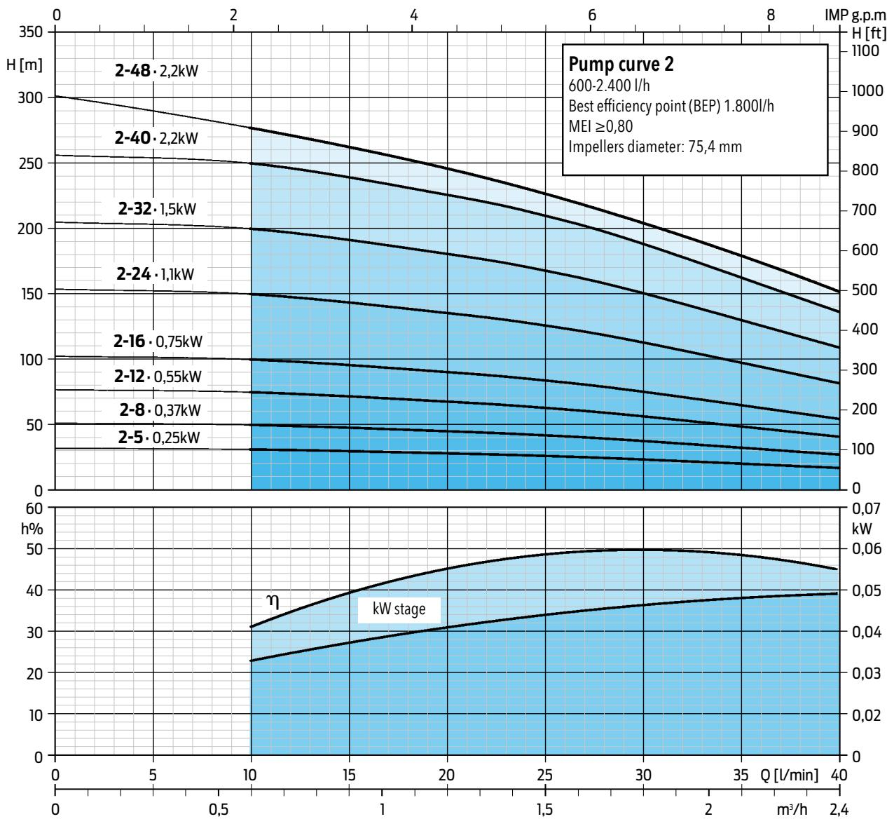
\* 4" NEMA standard dimensions • Operating curves at: 2850 min<sup>-1</sup> • Performance limits: ISO 9906 – annex A, mass production pump section.
